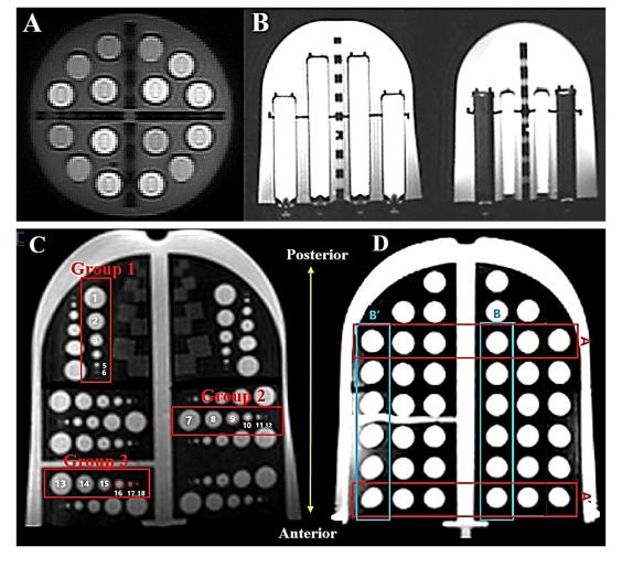
**Figure 2.** Method of ADC (A) and SNR (B) measurements on each representative slices using DWI phantom. Make five to ten ROI measured and derived mean ± SD (A) of ADC value. For SNR, an average of ROIs within each test tube devided by an average of ROIs in the background (B). The vendors were A, B, and C from left to right. Nyquist artifact was noted on vendor A image (asterisk on A and B).
