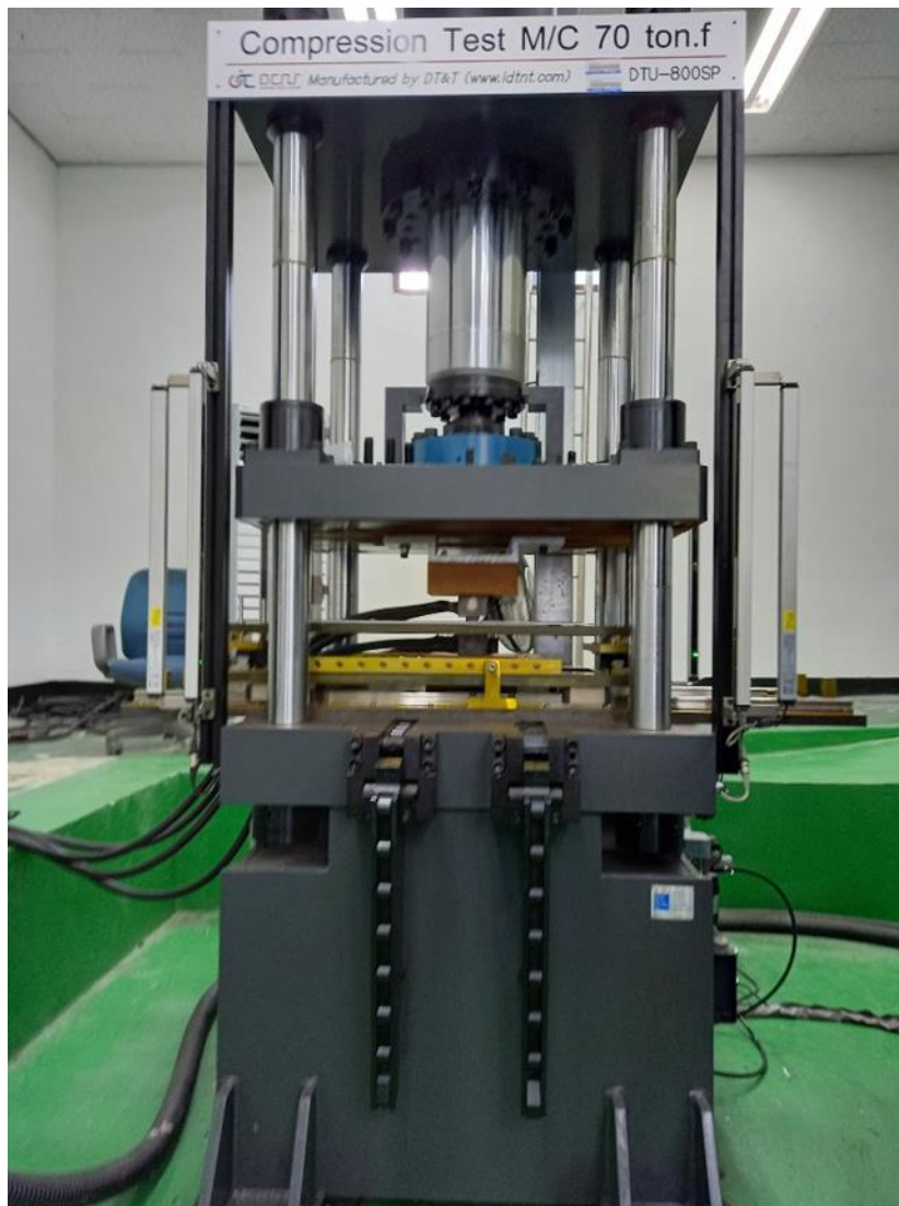
Fig. 5. 8. The experimental set-up for battery case joining by EAPJ
