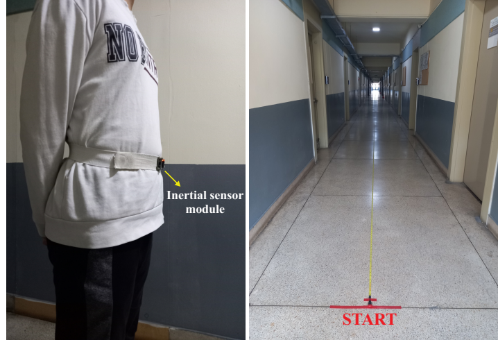
Figure 5-6: Experimental setup: an inertial sensor module is mounted on the user’s waist (left) and an indoor environment is designed to collect the training and testing data (right).
