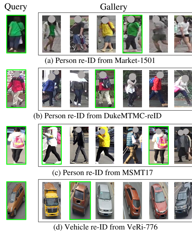
FIGURE 1.1: The examples of object re-ID images. Green boxes denote the matching identity between query and gallery.
