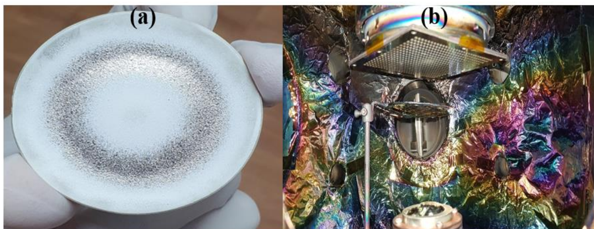
Figure 4.2. (a) Optical image of Silver (Ag) Target (b) Distance between the substrate and target in the RF magnetron sputtering chamber
