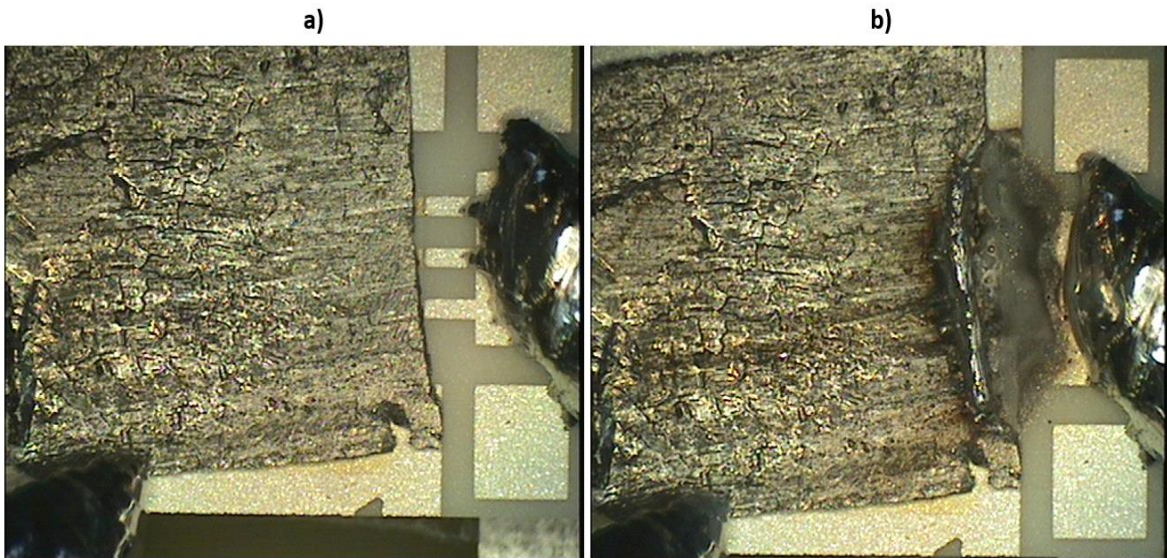
Figure 5.6. Triode micro fuse device blown at 5A applied current (a) before applied current (b) after applying the blown fuse
