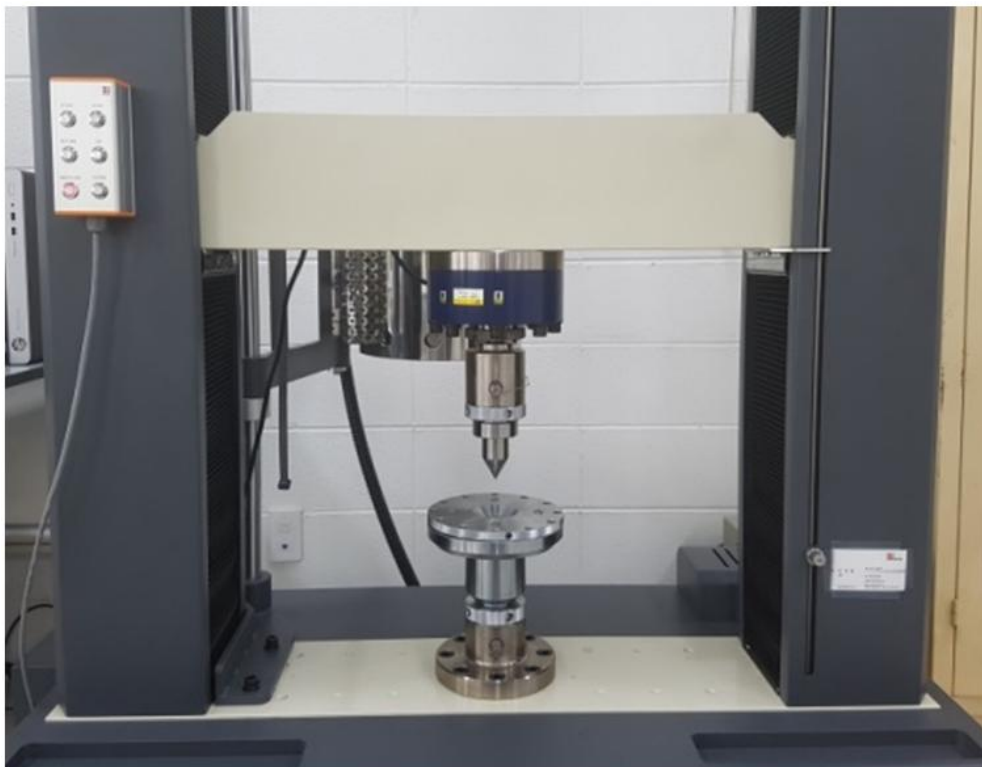
Figure 3 - 2 Hole expansion simulation test.
