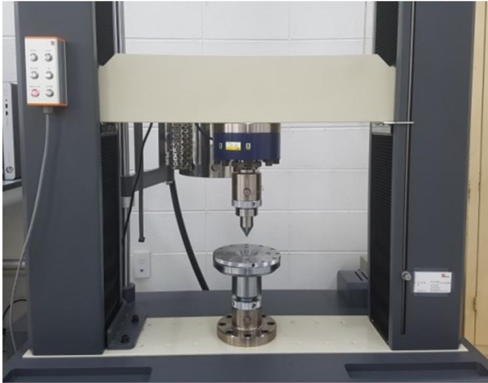
Figure 3-2 Hole expansion imitation test machine.
