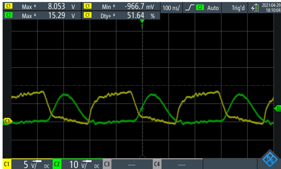
Figure 5.19 Drain voltage (green) and gate voltage (yellow) of the RF amplifier.
