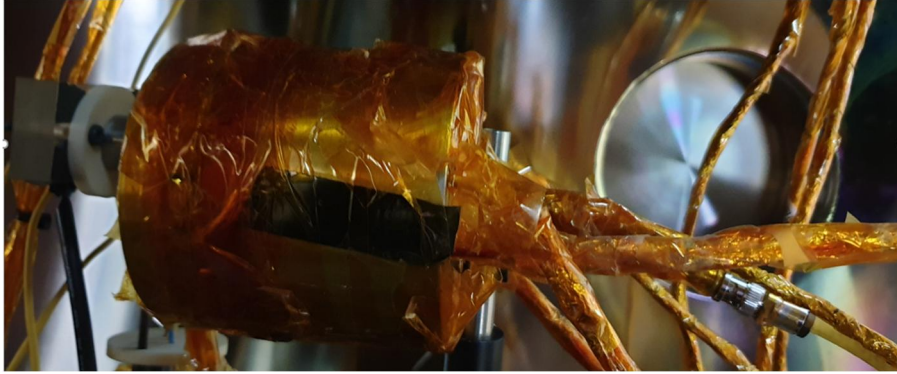
Figure 4.19 RF power supply system testing with RF ion thruster in the vacuum chamber. 1) RF generator; 2) Directional coupler; 3) Electrical feedthrough.
