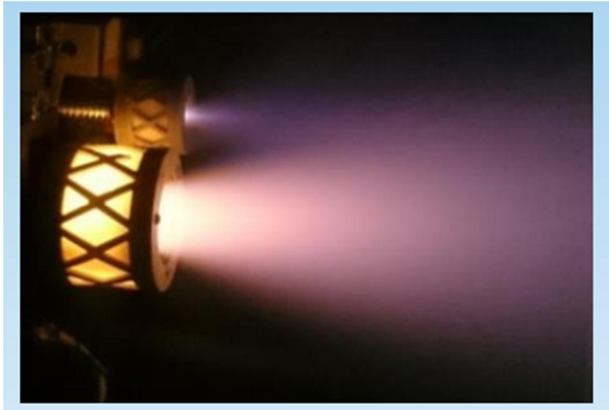
Figure 1.2 Prototype BIT-3 Thruster firing on iodine.
