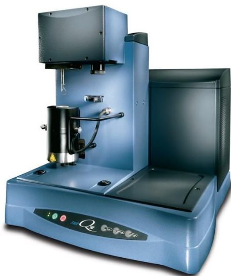
Figure 2.5. TGA instrument (Q50, TA Instruments, USA).
