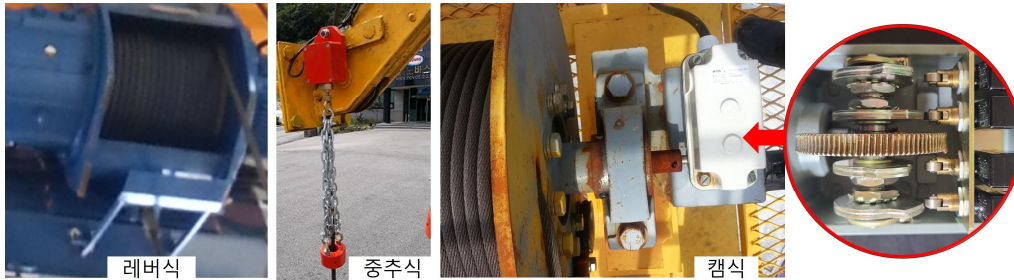
[Figure 15] 권과방지장치(upper limit)
