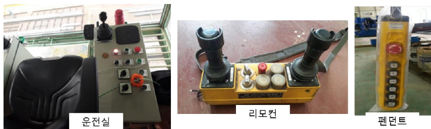
[Figure 12] 조작장치(operating device) (이용석, 2019)
