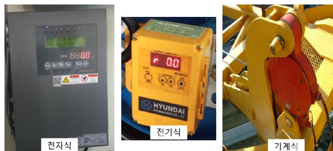
[Figure 16] 과부하방지장치(overload limiter) (이용석, 2019)
