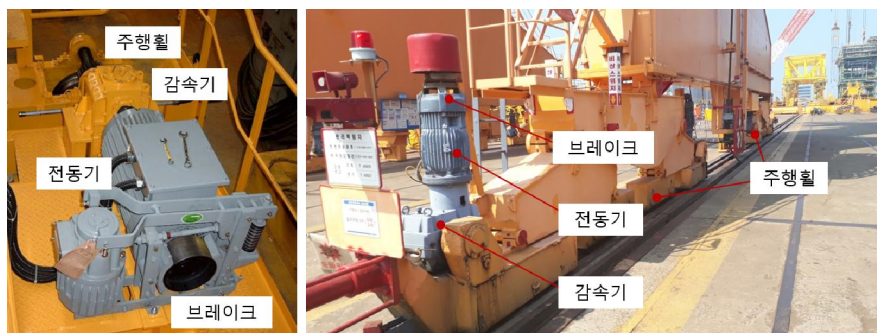
[Figure 11] 주행장치(travelling device) (이용석, 2019)
