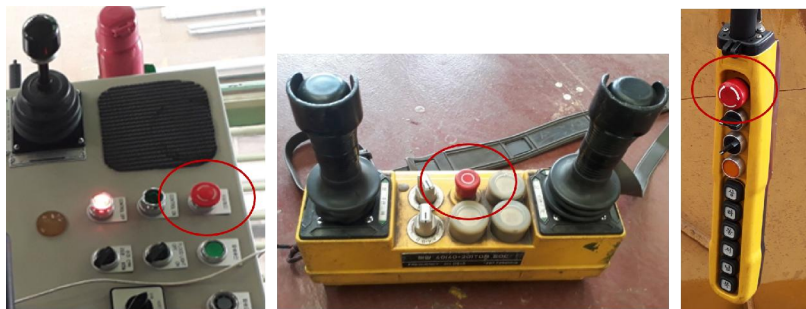
[Figure 14] 비상정지장치(emergency stop)
