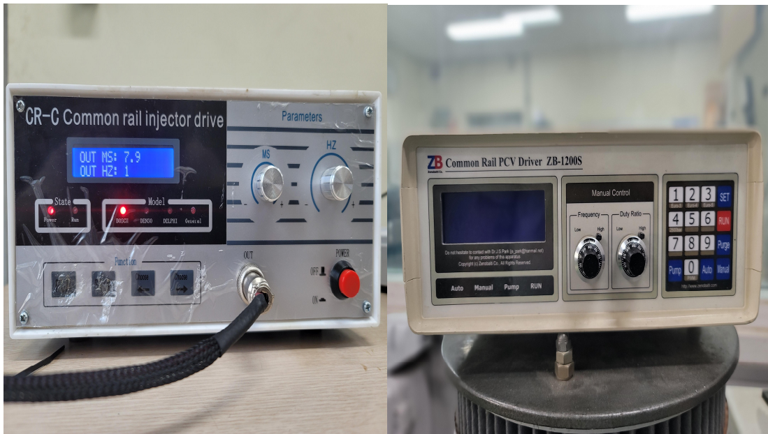
Fig. 2-10 Injector driver and PCV valve driver
