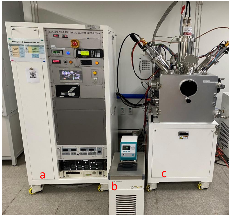
Fig 9. Ion milling system including a) power controller, b) cooling system and c) vacuum chamber at Department of Physics, University of Ulsan
