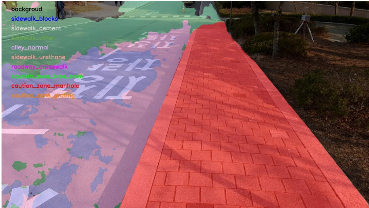
Fig 13. After label merging, the result of STDC2 trained on Korean Pedestrian dataset
