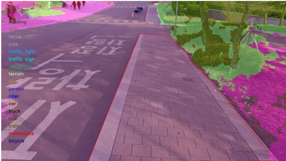
Figure 10. Inference Image with STDC2 trained with CityScapes dataset on Korean pedestrian environment
