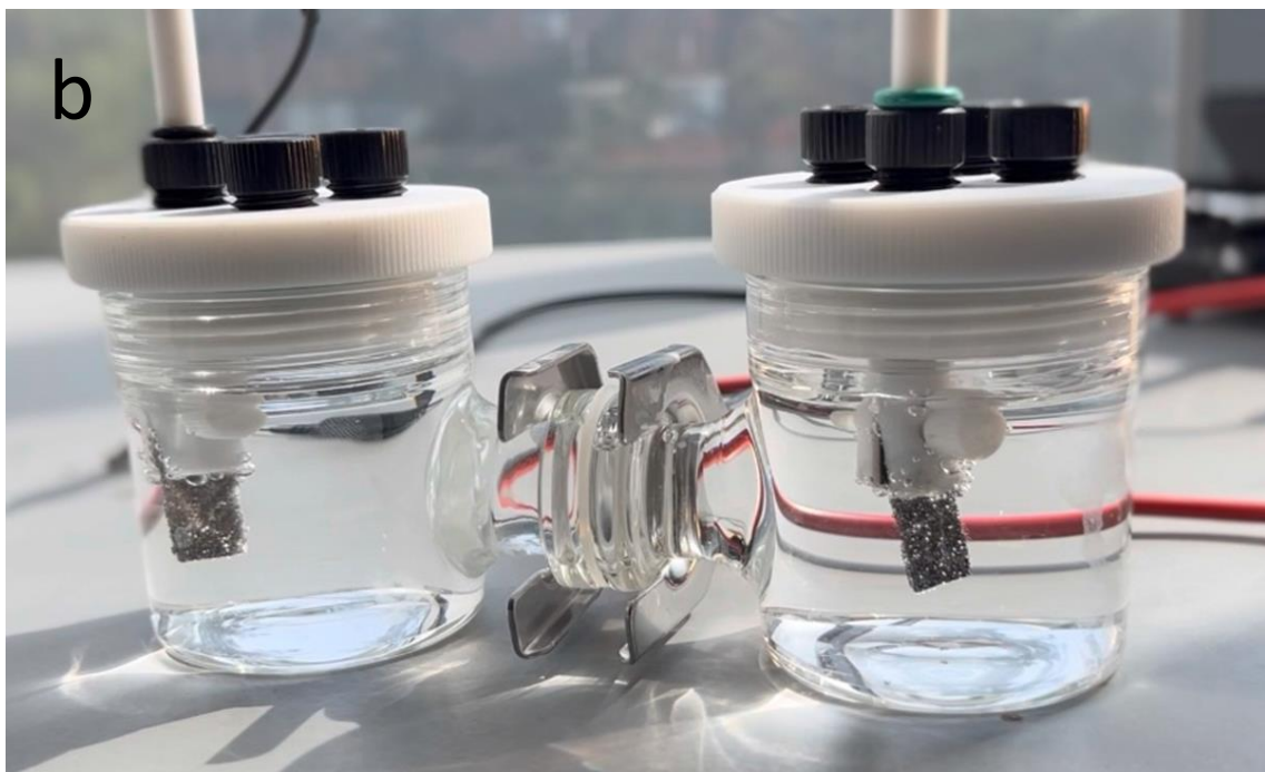
Figure 2.13: (a) OWS working by solar system, (b) 2 electrode in OWS
