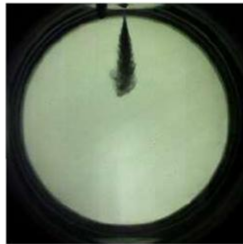
Figure 1.2 Non-reactive fuel spray in inert atmosphere using single hole fuel injector
