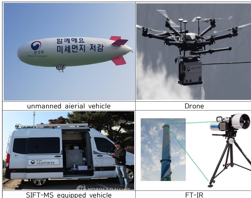
Fig. 1. Real time VOCs measuring equipment
