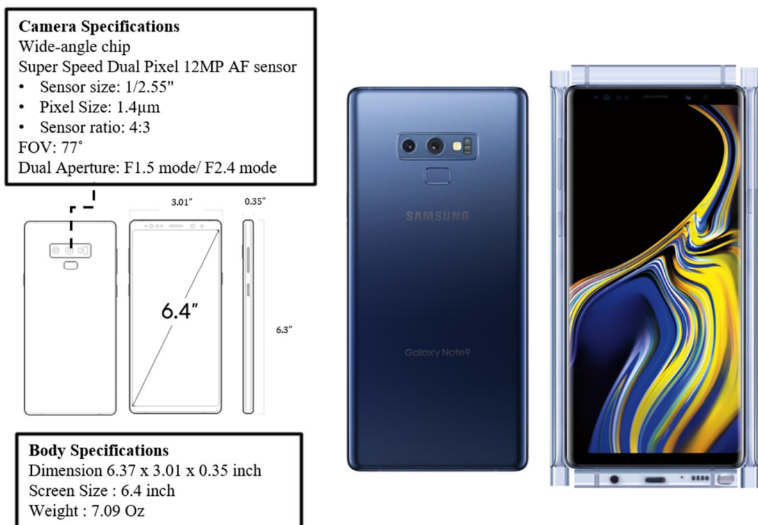
Figure 5. The image and specifications of the smartphone model (Galaxy Note 9, Samsung) used in developed smartphone-based endoscope device
