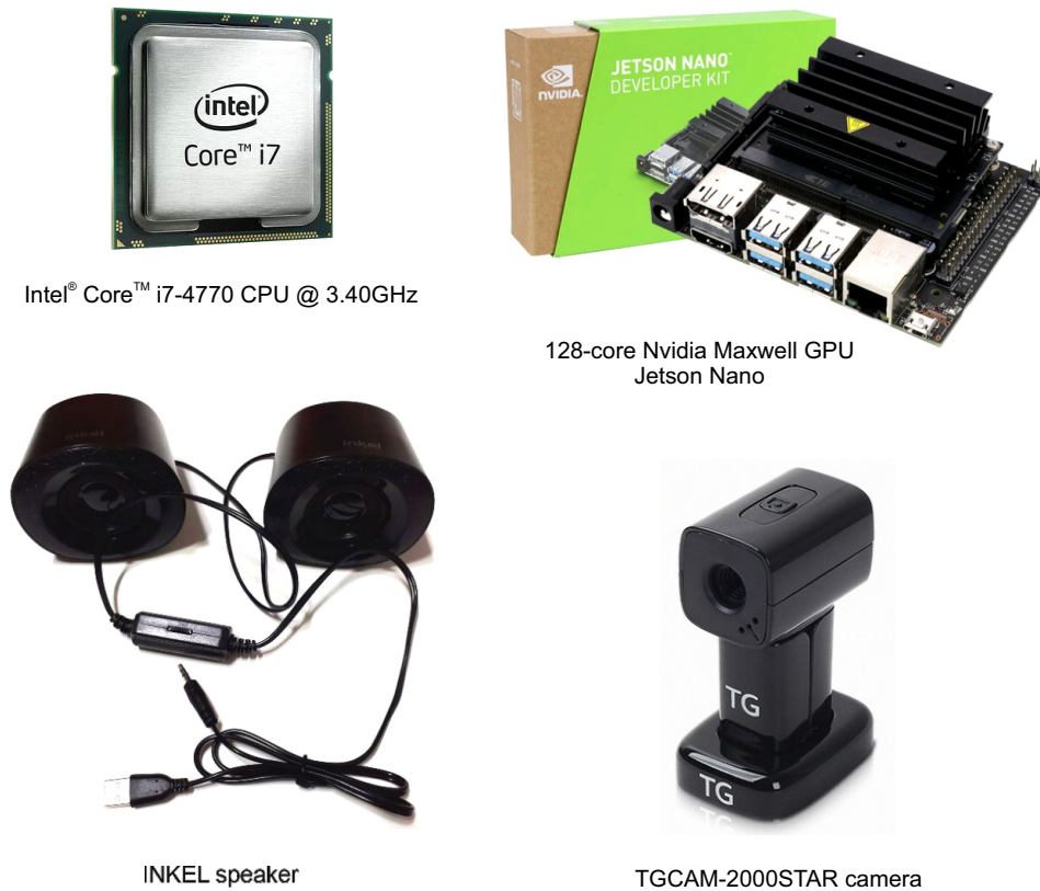
FIGURE 5.3: The hardware is used in the real-time eye status monitoring system.
