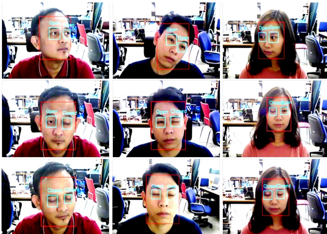
FIGURE 5.5: The qualitative results of the real-time eye status monitoring system with VGA video live-stream on Jetson Nano device with three participants.
