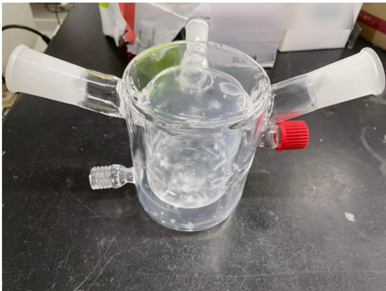
Figure 47. Quartz flask reactor (300 mL, diameter: 70 mm, and height: 80 mm), side view.
