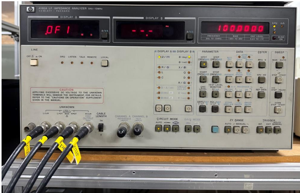
Figure D.1 Experimental set-up of the temperature-dependent dielectric constant. A HP4192A analyzer was used to measure dielectric permittivity as a function of temperature.
