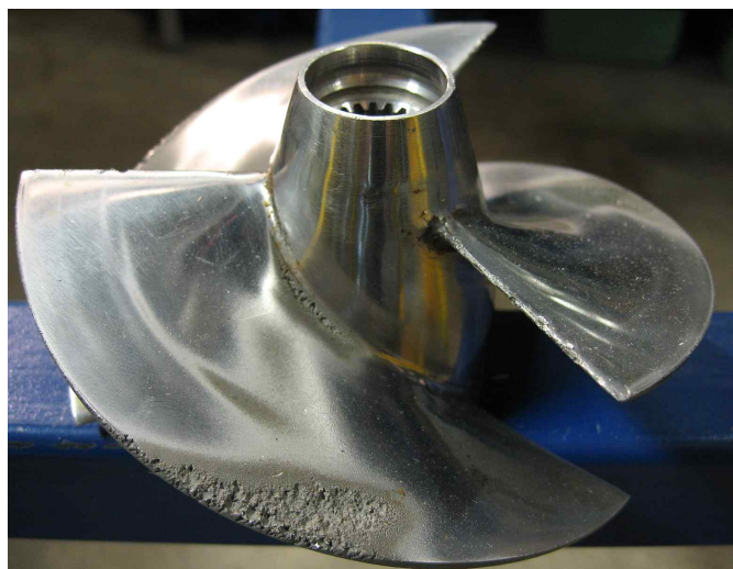
Figure 2 Propeller damaged by cavitation
