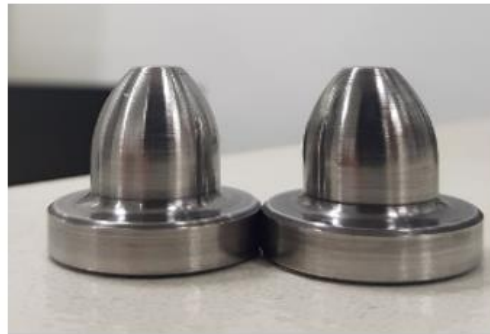
Fig. 11. Dimension and shape of electrode
