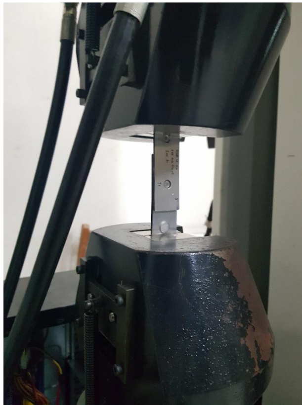
Fig. 19. The shear tensile test on universal tensile testing machine
