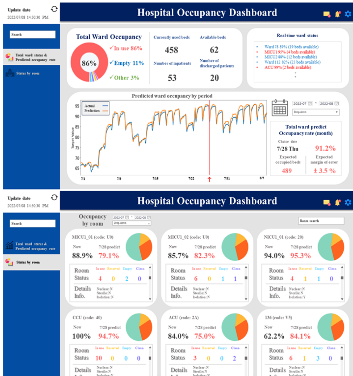
Figure 1. A virtual dashboard of the status and forecast of WBOR and RBOR. (1) On the first screen, the overall BOR of the hospital is shown, along with the number of beds in use and available. Moreover, a predictive graph displays the anticipated WBOR for selected dates. (2) The second screen presents the WBOR for individual beds, indicating their statuses such as “in use,” “reserved,” “empty,” and “cleaning.” Detailed information about each room is also displayed
