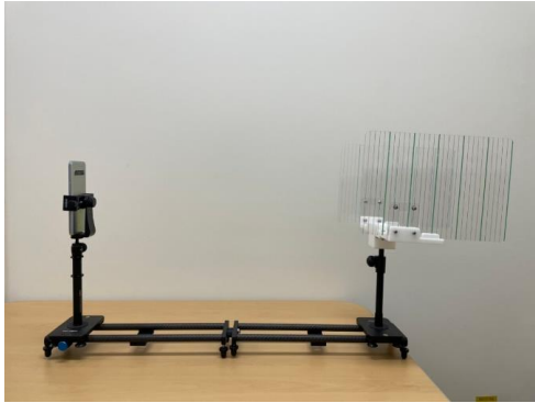
Figure 1. Composition of the frame. (A) The frame was composed of a phone holder on one side and a chin rest on the other. The distance was fixed with a bar. To confirm a neutral position, markings were placed bilaterally next to the chin rest, (B) The heights of the phone holder and chin rest could each be individually adjusted for the patient.
