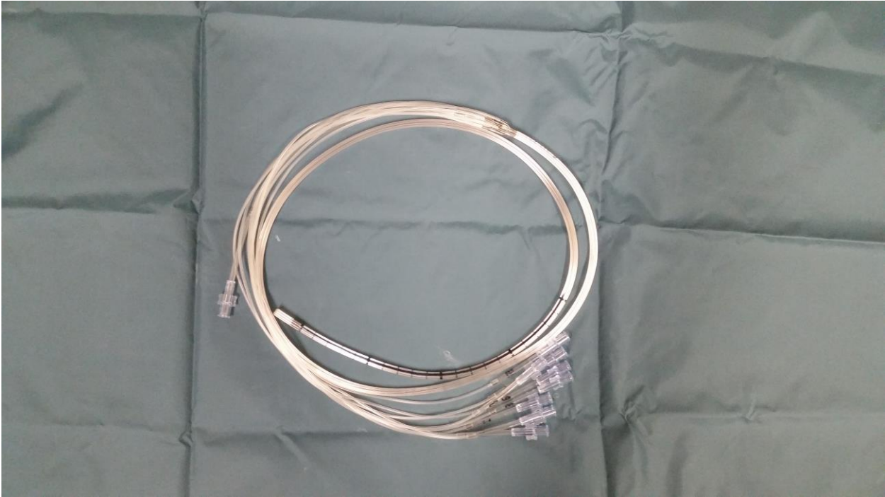
Figure 2. The pressure-measuring catheter with eight radial pressure measuring channels.
