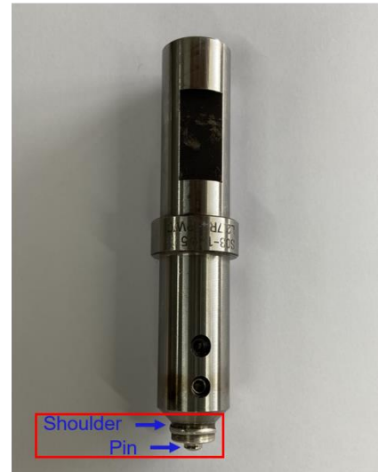
Figure 3-1 (a) Schematic diagram of FSW tool, (b) FSW tool
