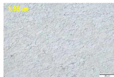
Figure 4-2 lower sheet panorama and microstructure of FSSW sample joints with plunge depth of 0.7 mm, 0.8 mm, and 0.9 mm
