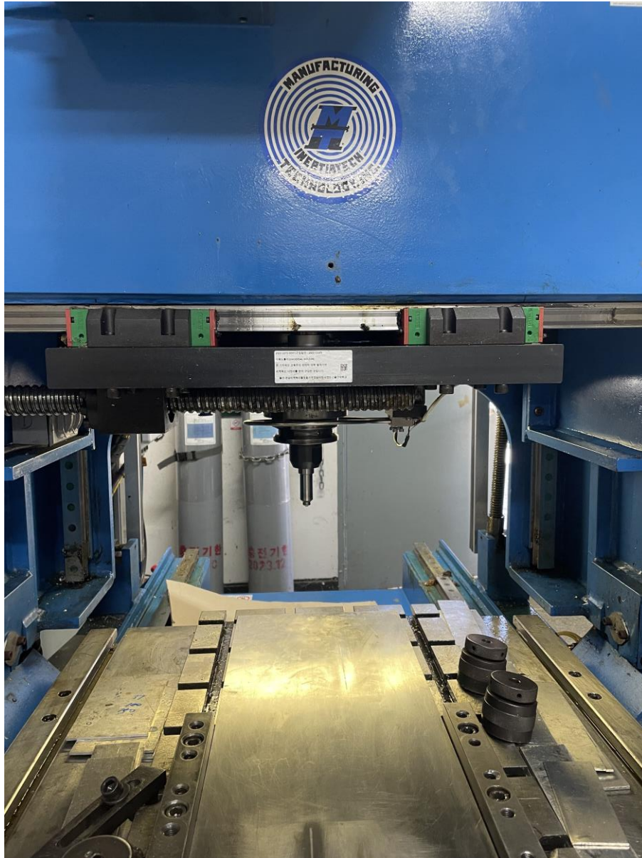
Figure 3-2 RM-1 FSSW machine made by Manufacturing Technology Inc.
