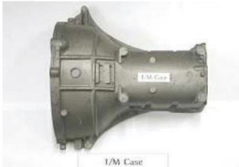
Figure 2-1 Cluth housing and transmission case inside body made of magnesium
