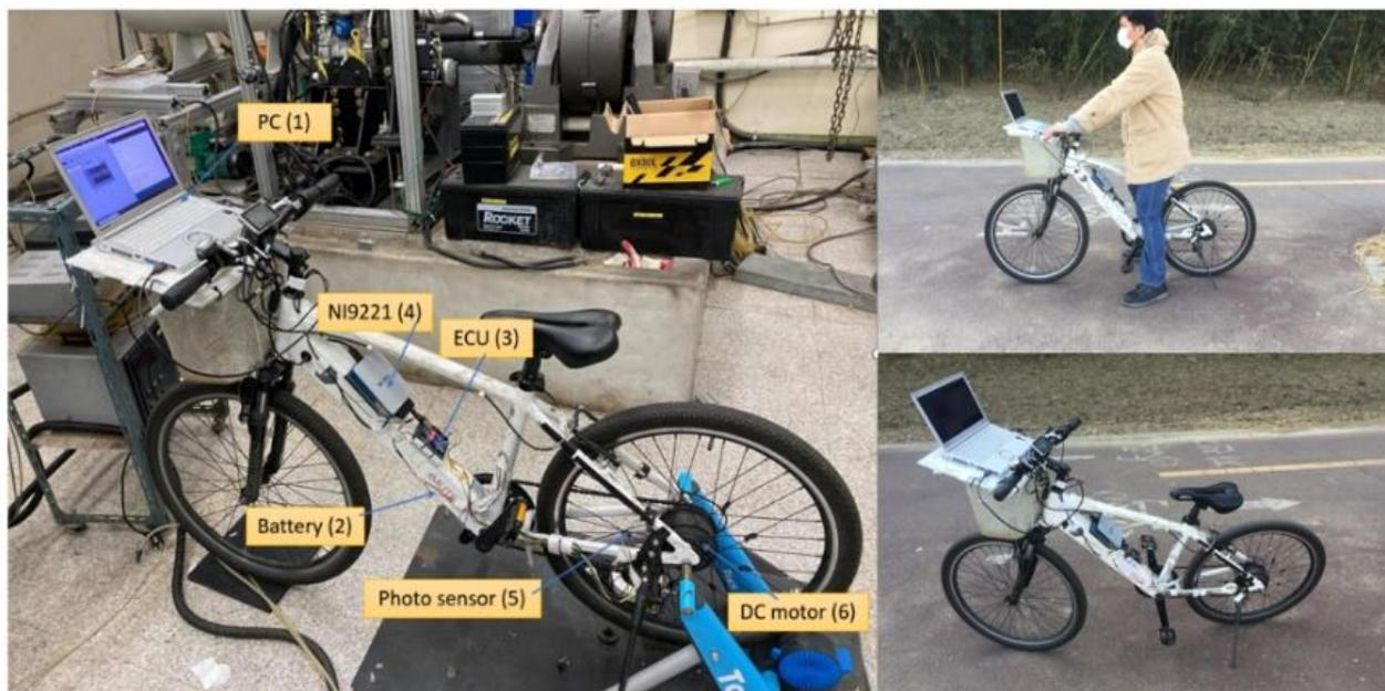
**Fig.3.1** Experimental system of an electric bicycle
