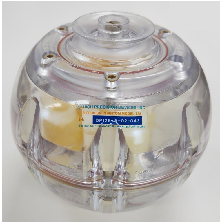
Figure 2. NIST/QIBA diffusion phantom
