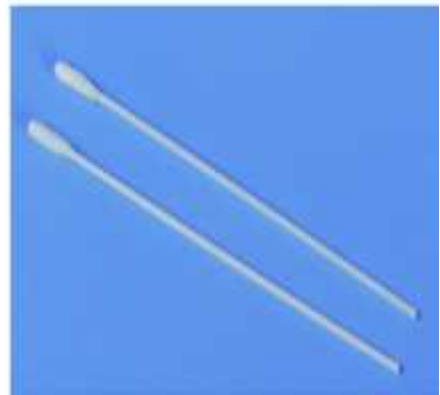
Figure 1. Types of swabs used in environmental surface sampling. flocked nylon and cotton swab (1-A), rayon swab (1-B)
