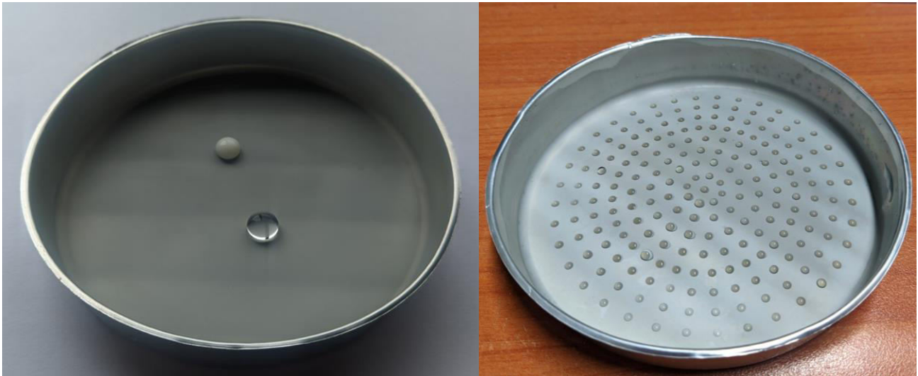
Figure 17: Superhydrophobic and superhydrophilic surface fabrication on a disposable aluminium dish.
