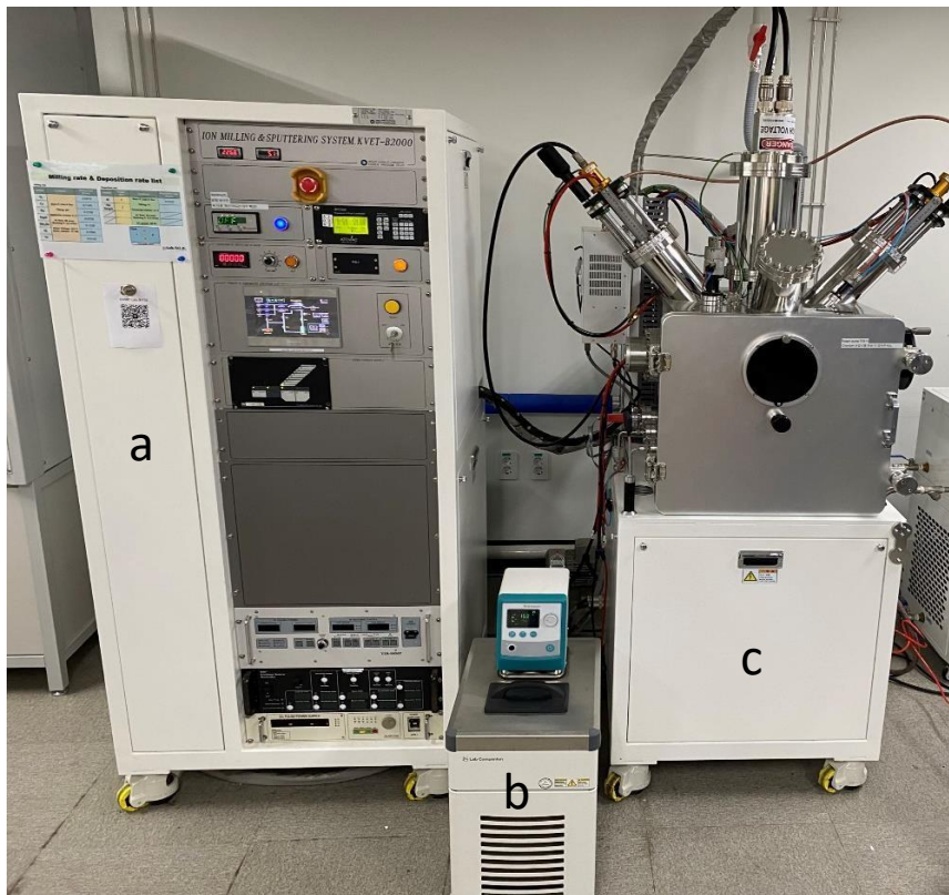
Figure 11. Ion milling system a) power controller, b) cooling system and c) chamber.
