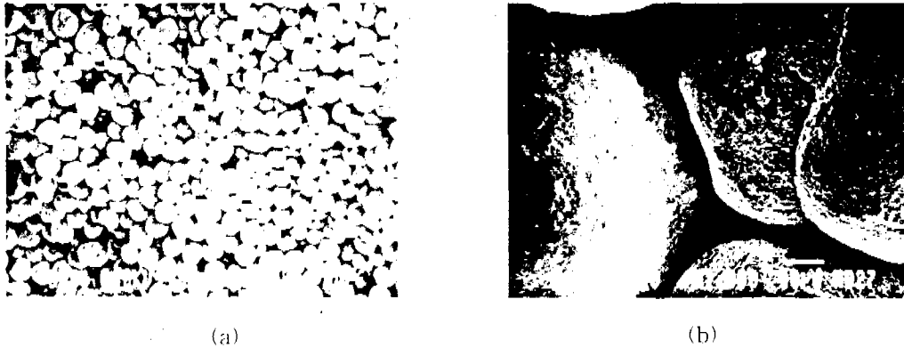
Fig. 6 SEM micrographs of (a) sintered Ni powder by SPS treatment, and (b) enlarged (a) [ Sintering condition : 86kgf/cm 2 pressure, 500°C, 5min ]
