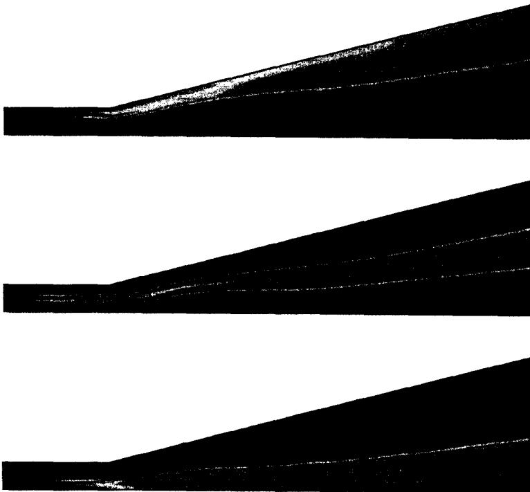
Fig. 2 Distribution of mass fraction of H_2O in three different cases: the fuels are located at (a) top (b) center and (c) bottom of the entrance plane, respectively. The maximum mass-fraction of H_2O is 0.06. The temperature of air and fuel is 817K and 1200K, respectively. The pressure and velocity of fuel are same with those of air.
