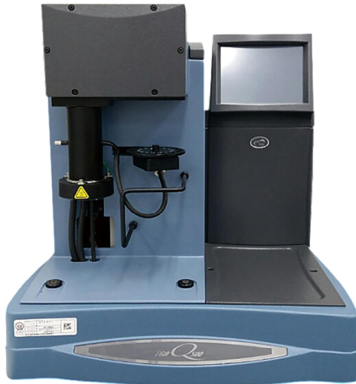
Fig 19. Image of TGA equipment <Model : Q500>
