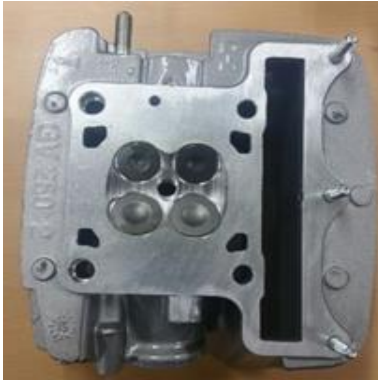
Fig. 3.1. Cylinder head of small gasoline engine
