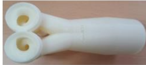
Helical intake port with opposite direction (inward) (model 2)
