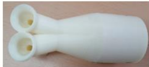
Tangential intake port (model 4)
