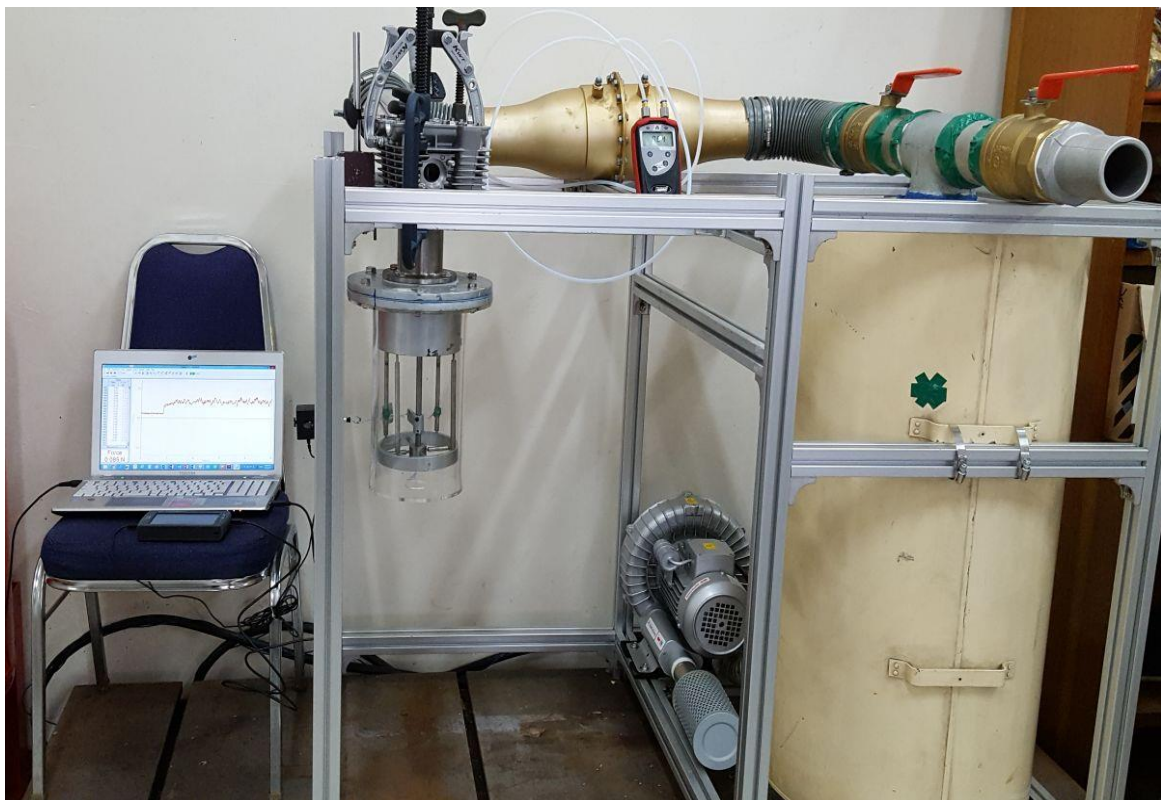
Fig. 3.8. Steady flow test experimental set up
