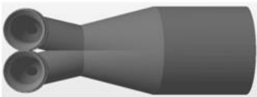
Tangential intake port (model 4)
