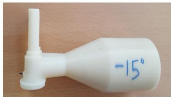
e. Intake port with -15^\circ
