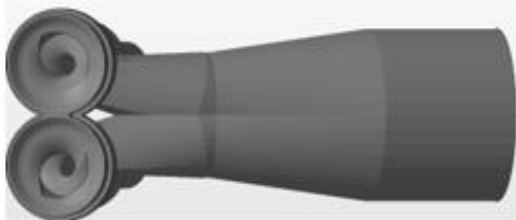
Helical intake port with opposite direction (outward) (model 3)
