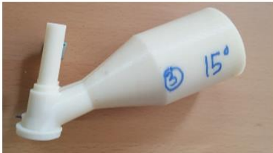
c. Intake port with 15^\circ
