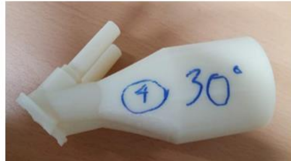
d. Intake port with 30^\circ
