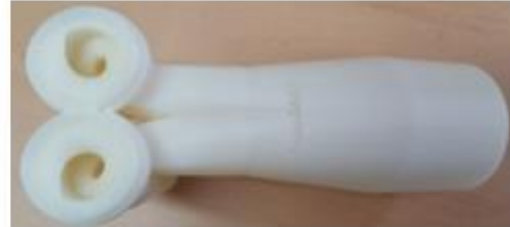
Helical intake port with opposite direction (outward) (model 3)
