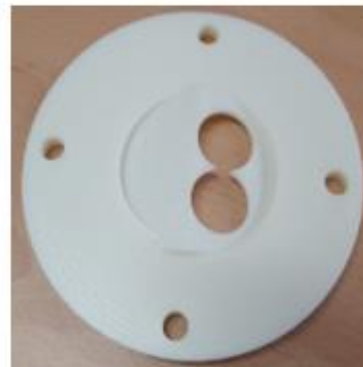
Body deck representing the bottom structure of the cylinder head
