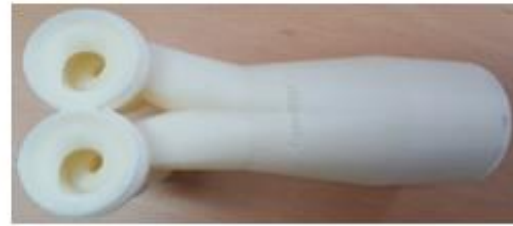
Helical intake port with same direction (model 1)
