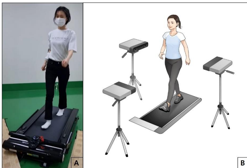
Figure 4. Experimental setup for motion tracking. The treadmill pointed directly toward the frontal depth sensor for the full-frontal plane view, and the others pointed to its side ( left arm, right arm ) orthogonally to the frontal camera centered in the treadmill.
