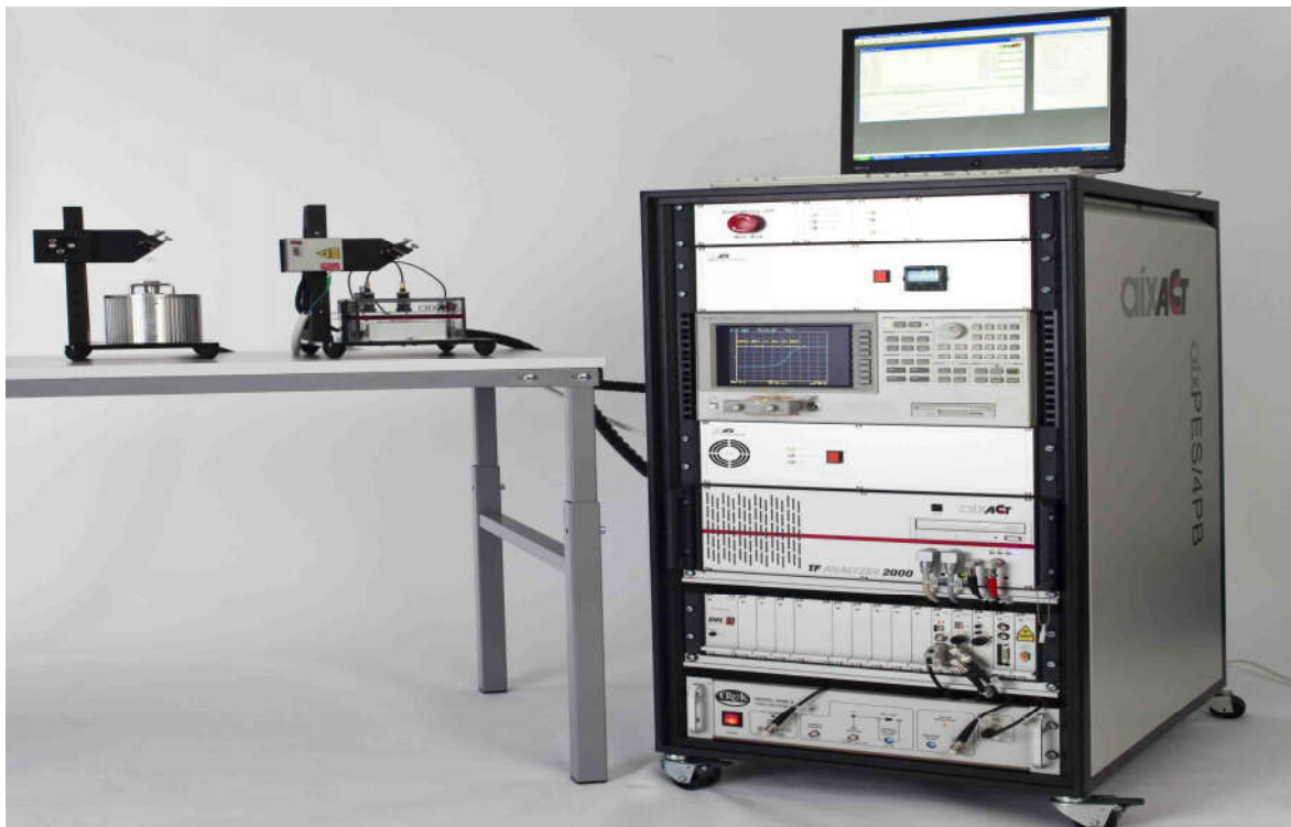
Figure 3.3. AixPES (aixACCT) setup for measuring P–E and S–E hysteresis loop.
