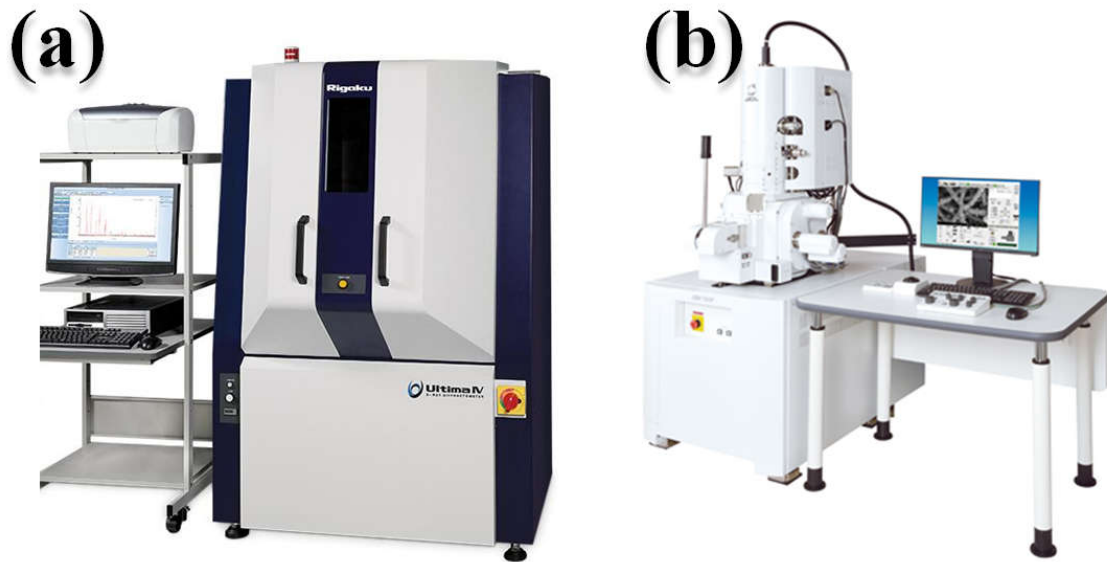
Figure 3.2. (a) Multi Purpose X-Ray Diffractometer and (b) JEOL Field Emission Scanning Electron Microscope.
