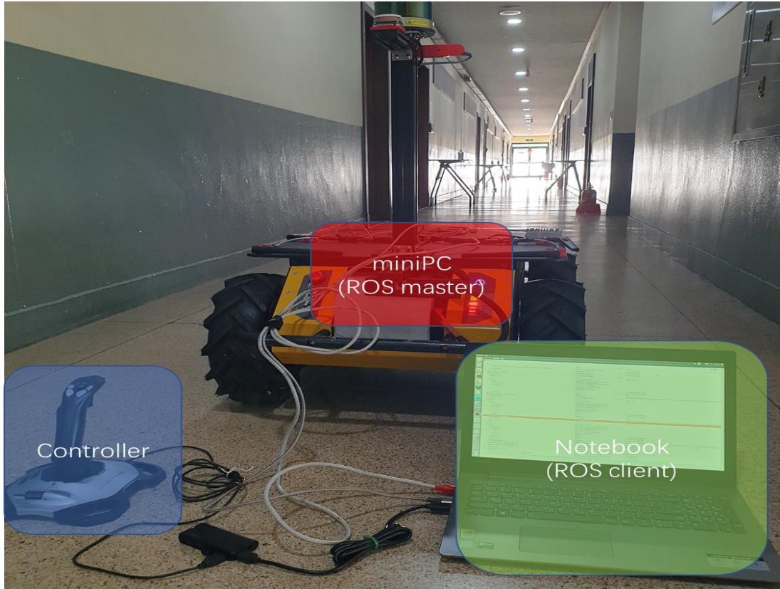
Figure 32 Controller and computing devices used in the experiment
