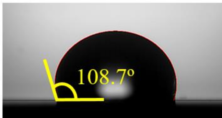
Fig. 3.5. Water contact angle of 510 nm ZnO on alumina
