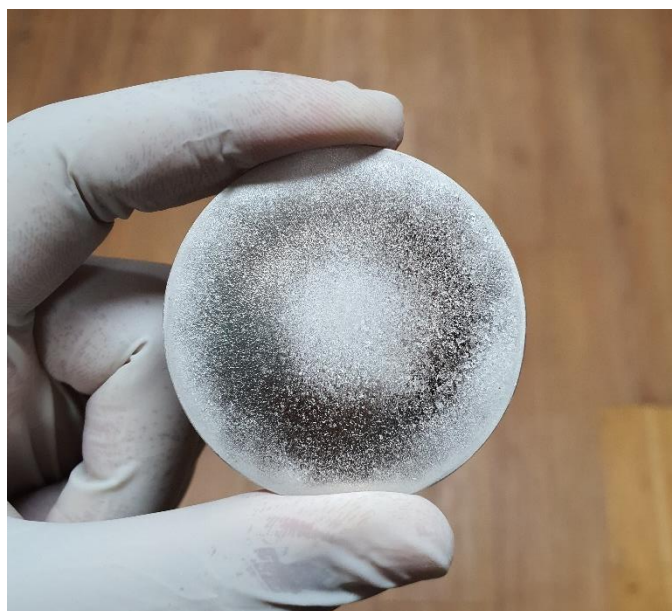
Fig. 3.7. Pt target (iTASCO, 99.99% purity)
