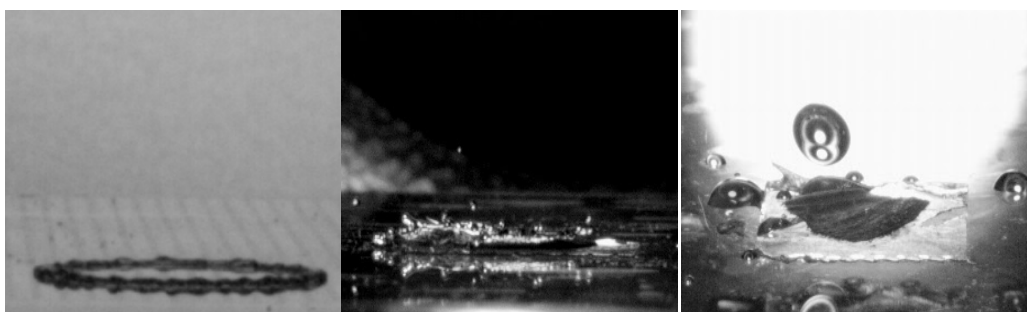
Fig1.1 Spreading (left) splash (middle) and bouncing (right) of droplets
