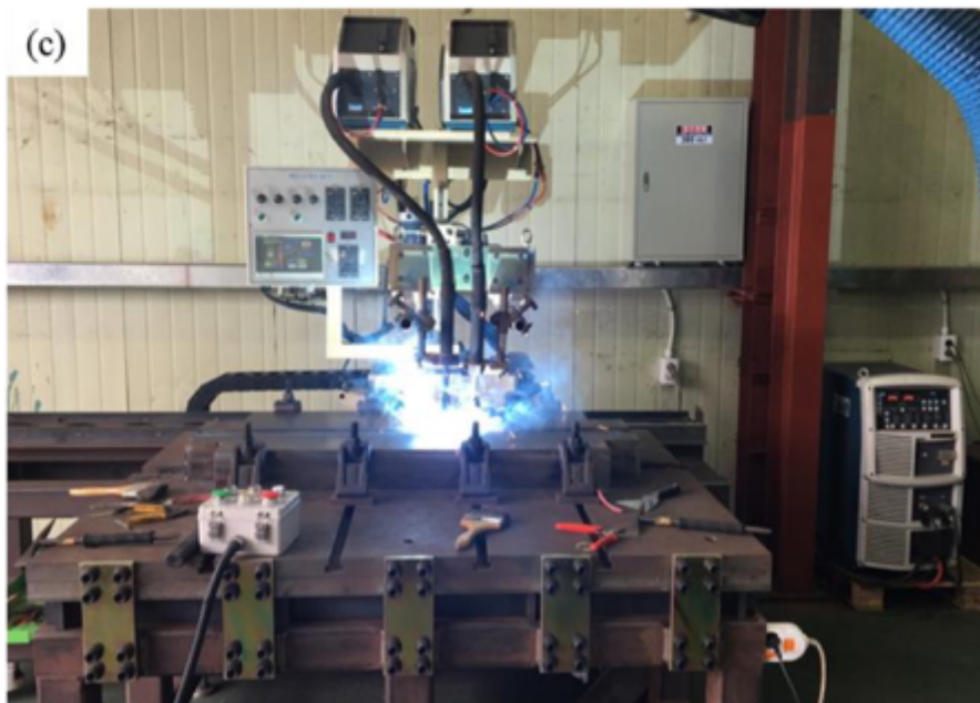
Figure 2-5. Schematic illustration of the flux cored arc weld: (a) overall process (b) welding area enlarged (c) actually FCA welding
