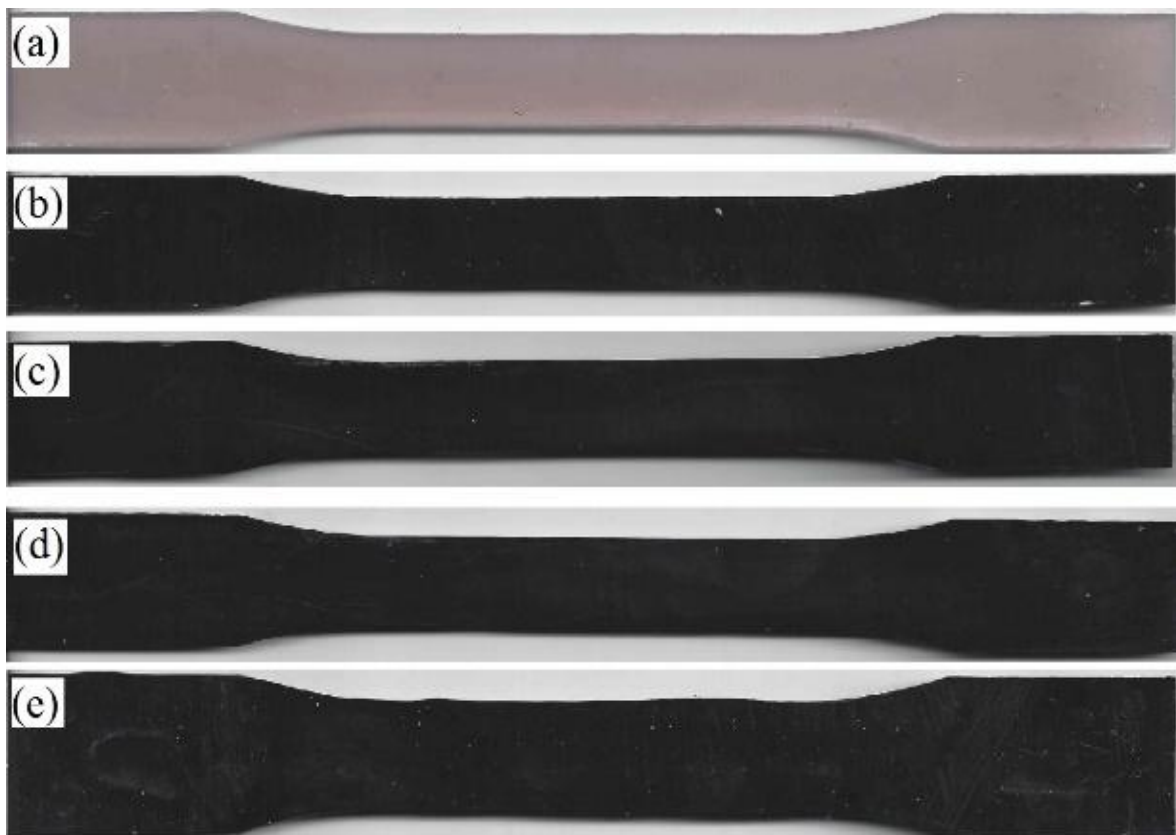
Figure 3-5: Dispersion of MWCNTs in UPR
