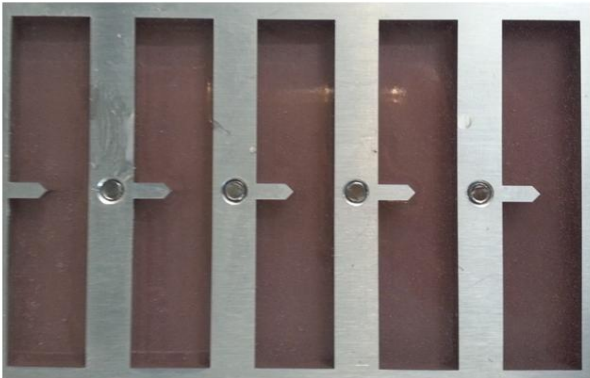
Figure 5-3: UPR after casting in aluminum mold
