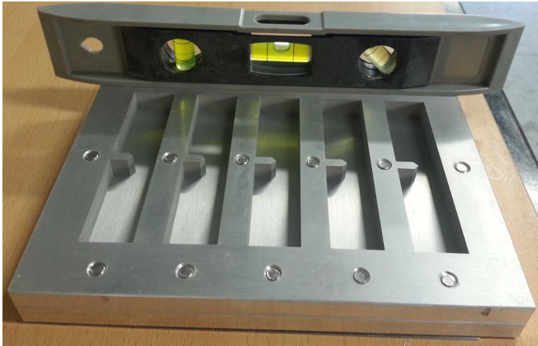
Figure 5-1: Aluminum mold for casting UPR
