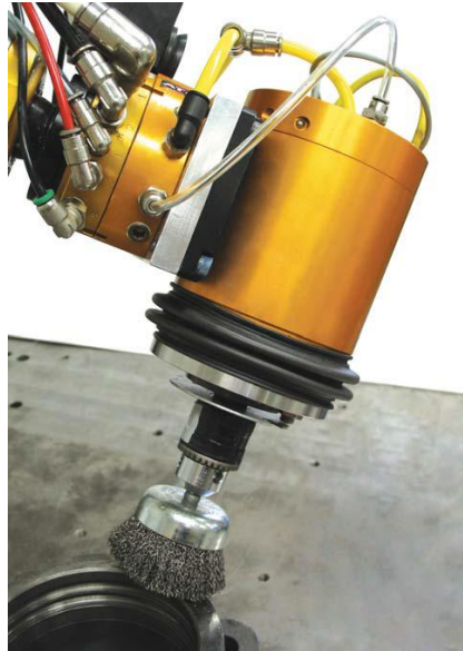
Fig. 17 An application example of a metal deburring tool.
