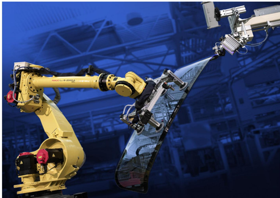
Fig. 9 Example of the transfer mechanism of vacuum adsorption.
