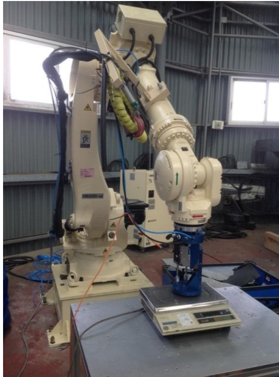
Fig. 40 Force Measurement Test using IDC Device.
