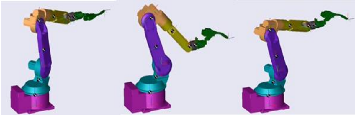
Fig. 37 Example of deburring robot modeling.
