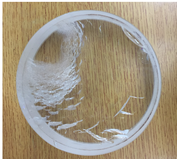
Figure 3.14: The quartz is broken due to the knocking
