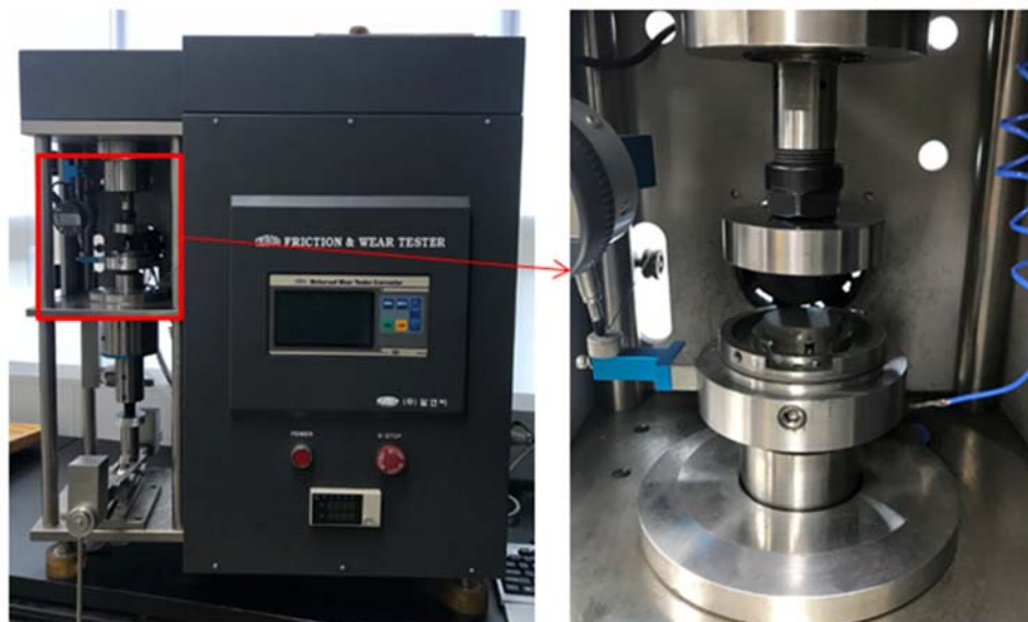
Fig. 5.2 Wear test equipment and test condition of wear test specimen
