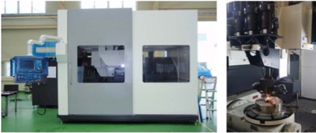
Fig. 4.1 DED equipment, (DMT 3D metal printers MX3, Insstek Co., Ltd.)
