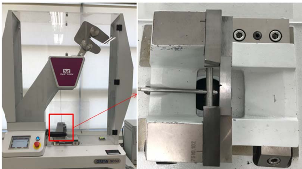
Fig. 5.3 Impact test equipment and mounting condition of impact test specimen
