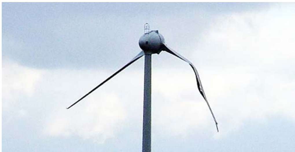
Fig. 4 Fatigue Failure of Wind Turbine Blades [12]
