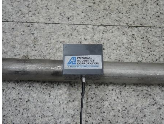
Figure 7.3 The AE sensor mounted with the magnetic hold down and vacuum grease couplant.
