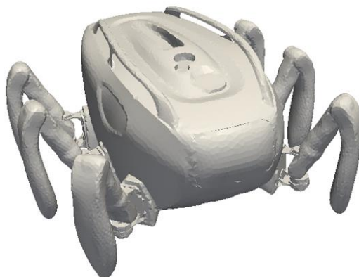
Fig. 4.18. The rendered surface of the underwater walking robot “Crabster”. Crabster is a bio-inspired underwater robot which consists of a main body and six legs. This 3D geometry is composed of 49,400 triangular surface meshes, and its original geometric information is provided by the Korea Research Institute of Ships and Ocean Engineering (KRISO) [108].
