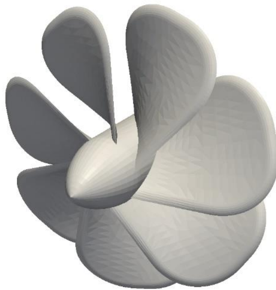
Fig. 4.15. The rendered surface of 3D propeller that consists of 7-blade and cone shaped hub. This 3D geometry is composed of 14,480 triangular surface meshes, and it is downloaded in online design community GrabCAD ( https://grabcad.com/library/propeller-airplane-1 ).
