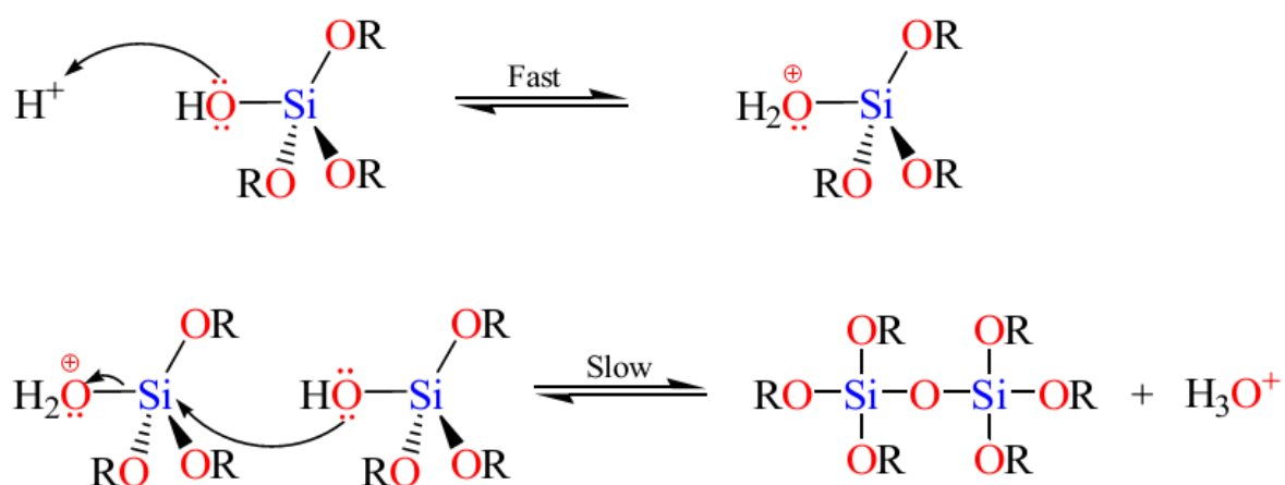
Figure 2-12: Condensation mechanism of an alkoxy silane using acidic catalyst [35].
